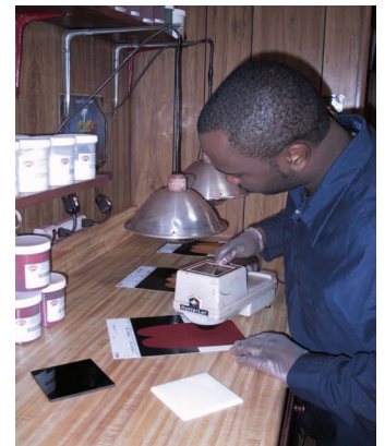
Charles with the Hunter Labs Spectrophotometer comparing color formulations in APC Color Lab.
